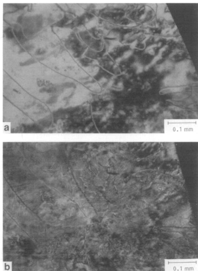
Figure 8 Threaded texture of the nematic phase at 130°C (a) and texture of the smectic phase (b) after annealing during one night at 85°C. Crossed polarizers. Run 5
